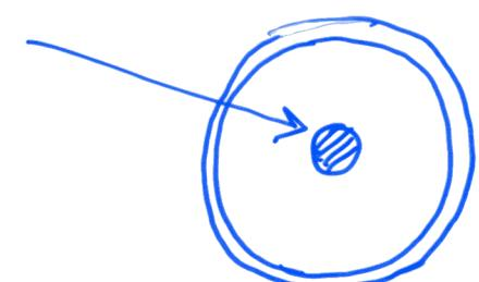
Ring in homogeneous field:  $\Phi = \pi R^2 H$
